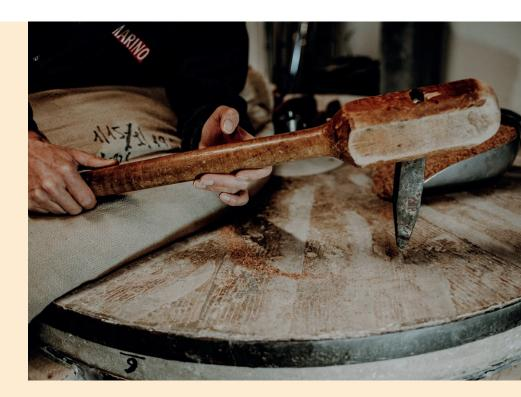
Our mill stones need to be periodically hammered by hand to create the right surface for milling each type of cereal.
